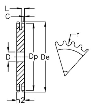
C = 4 D = 40 De = 524.7 Dp = 509.85 For chain size = 1 1/2 x 1 For chain type = 24 B-2
